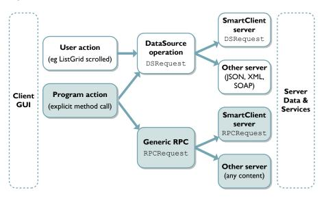
RPC operations sent to the SmartClient Java Server can use DMI declarations to route requests to appropriate server-side code, or a custom servlet can interact with the server-side RPCManager class to receive the RPCRequest.
